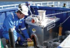
we serve. We also conducted our first automated ultrasonic (AUT) pipeline inspections for customers in West Africa and the Middle East. Due to enhanced productivity on offshore pipelay barges and inherent safety advantages, we expect continued growth in the use of AUT technology in 2008 and beyond.
