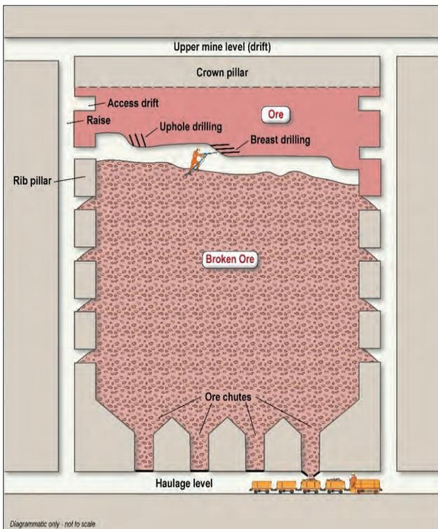
Diagram 3: Schematic diagram of a shrink stope
