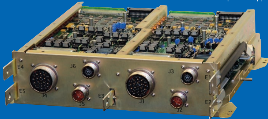
Electronic Power Distribution Center for Small Business Aircraft
