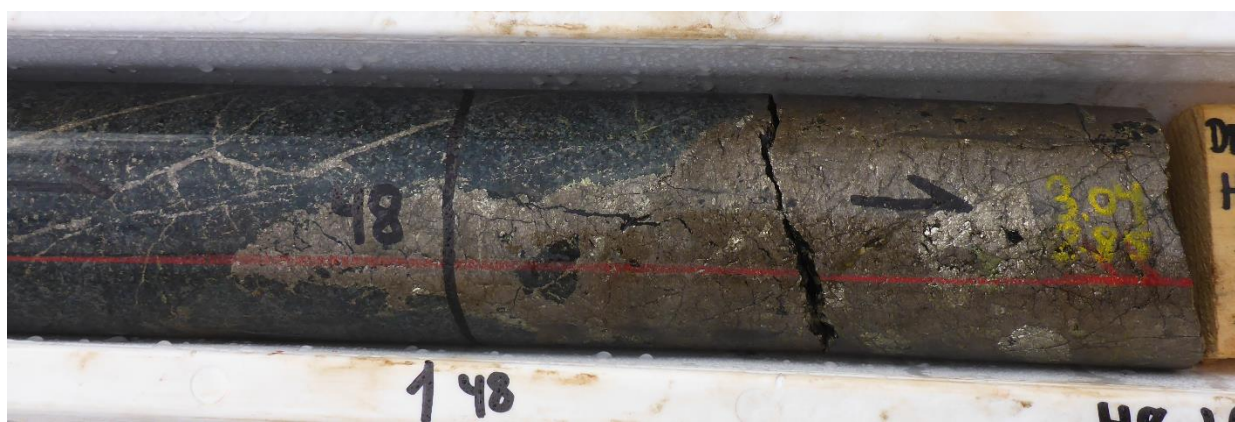
Figure 5 – Close up core photo of irregular top contact of massive sulphide vein in DMDD0004 at Conductor D. Interval (0.5m downhole) assayed 8.14% Ni. Note core is HQ3, with a diameter of ~61.1mm.
