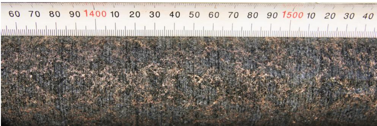
Figure 5 – Net-textured or matrix Ni-Cu sulphide mineralisation in Ruins Dolerite intercepted in DMDD0014, photo is of uncut HQ core, 311.40m to 311.60m downhole
