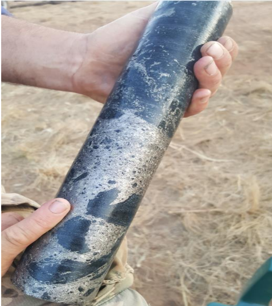
Figure 4 – Brecciated massive sulphide mineralisation in Ruins Dolerite intersected in DMDD0014, photo is of uncut HQ core, 318.5m to 319m downhole
