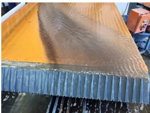
Figure 5: Separation process in action (with noticeable dark hue to the left indicating the presence of descloizite).
