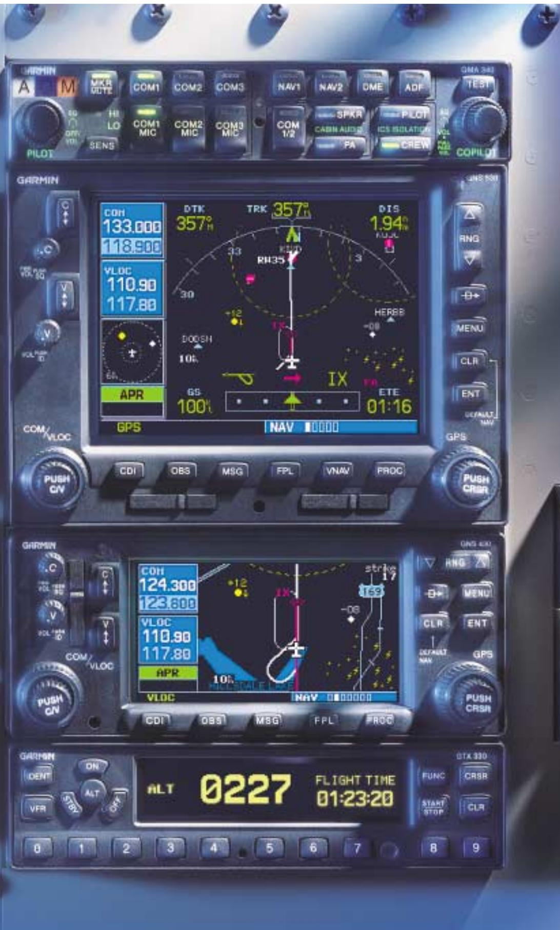
Garmin's avionics "stack" featuring the GMA 340 audio panel, GNS 530, GNS 430 and GTX 330 transponder
