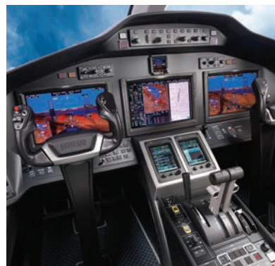
Cessna Latitude with Garmin G5000® avionics system
