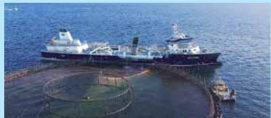
The technology is more robust than ever – a specialised offshore power management system has been fitted to the *Ronja Storm*, the first in a wellboat, which reduces energy use and noise emissions. The vessel includes backup power systems that ensure it can continue to operate with a minimum of 50% power capacity in case of system failure. This is essential in delivering robust, secure fish welfare practices.
