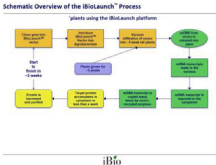
Subsequent to the incorporation of the iBioLaunch vector in the plant tissues, the following steps lead to target protein synthesis:
