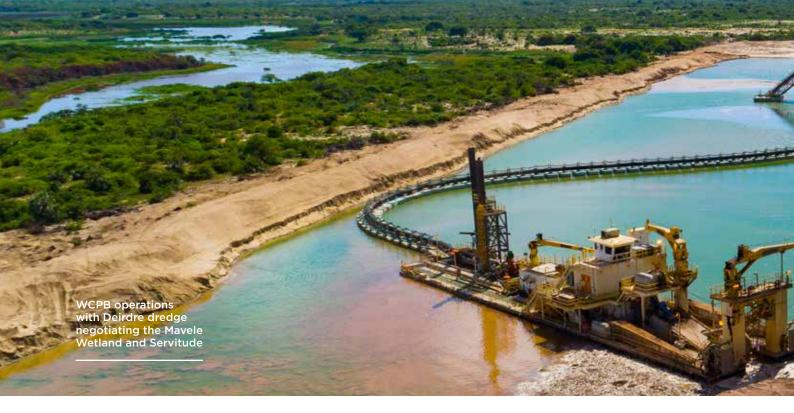
Kenmare first began production at Moma in 2007 and has built a high level of specialised expertise in dredge mining, a low-cost method of extracting minerals that is well suited to the deposits in which we operate. Throughput can be affected by variations in the levels of slimes, the hardness or softness of the ore and the height of the dunes being mined. Over time we have developed the experience and skills to efficiently mine and more accurately forecast the impact of these fluctuations.
