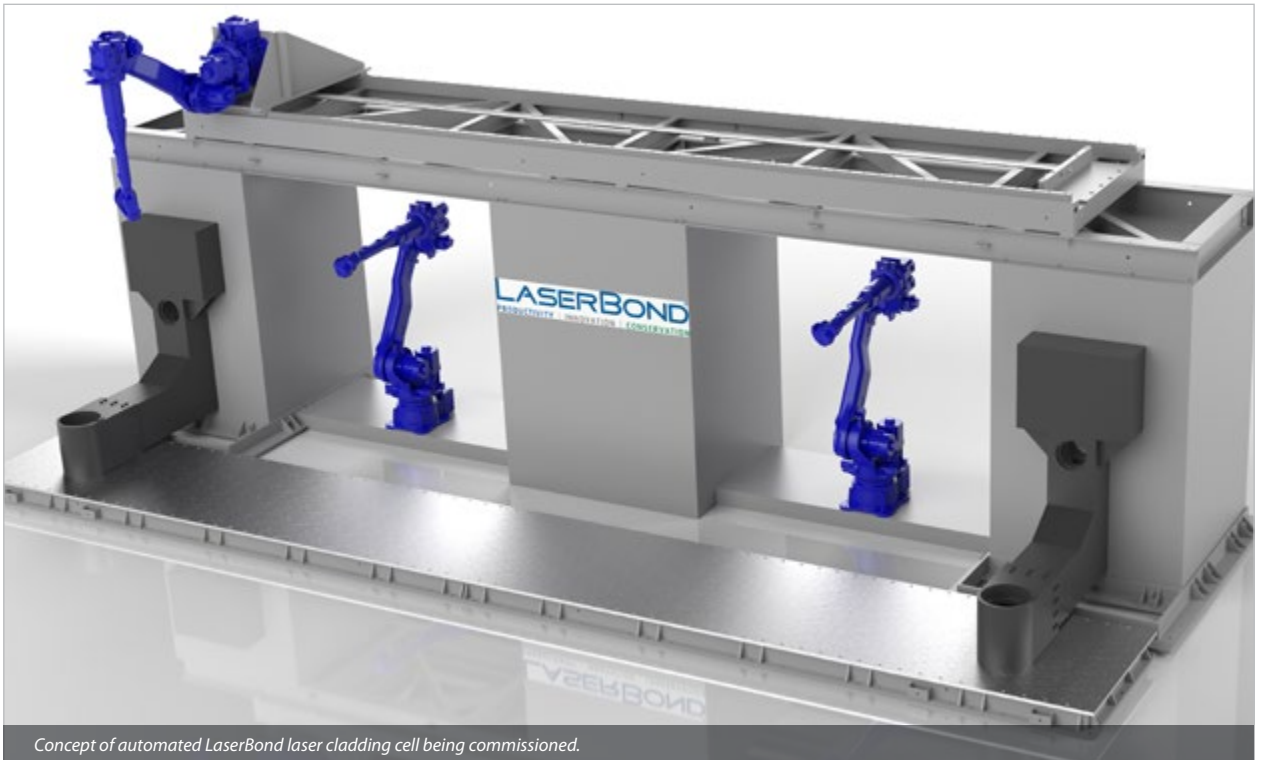
Concept of automated LaserBond laser cladding cell being commissioned.
