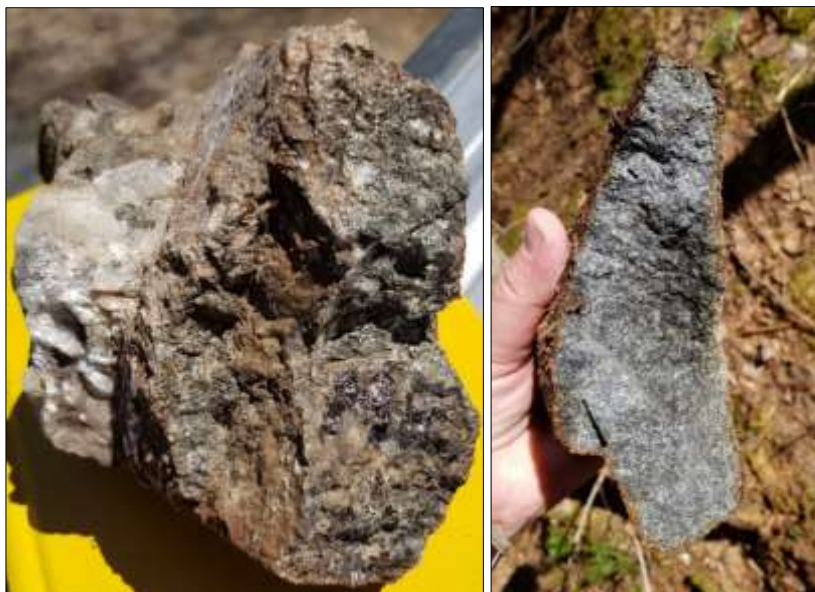
Figure 7: Quartz veining in Nipissing Diabase (left) and Nipissing Diabase hosting sulphide mineralisation (right)
