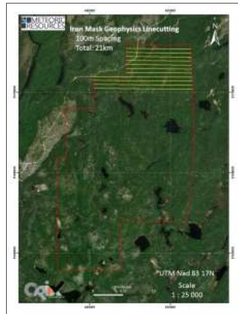
Figure 2: Iron Mask Cobalt Project 100m line spaced ground-based IP/Magnetics/Resistivity geophysics program. The program is due to complete in September with results expected in early October.
