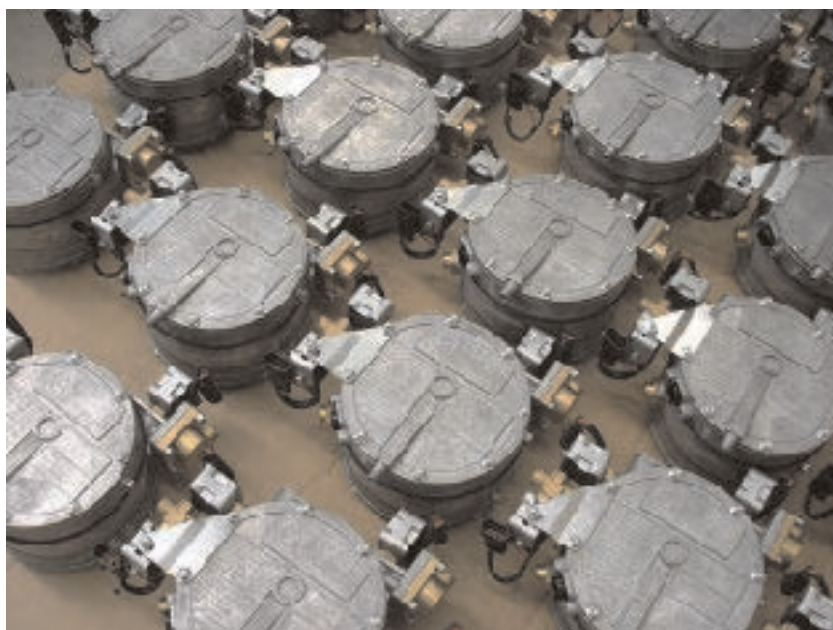
• Fuel metering units manufactured by Vialle for integration into Orbital Gas Product's LPG system.
