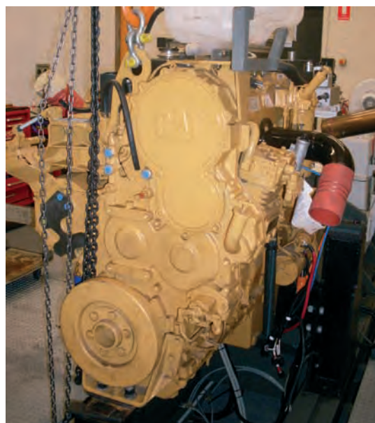
Installing a 15 litre engine in Orbital’s recently commissioned heavy duty engine test facility
