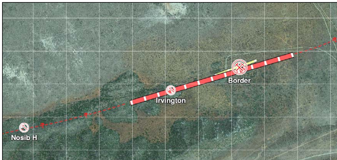
Figure 16 – Diagram showing the extent of visible lead and zinc sulphides at Border and Irvington. The previously defined extent (650m) at Border is shown in pale green. The present extent (2500m) is shown as a red bold line. Mineralised zones are open to the east and west. To the east, soil cover obscures mineralisation. To the west, more mapping is required, but mineralisation could conceivably extend to Nosib H prospect (500m grid).
