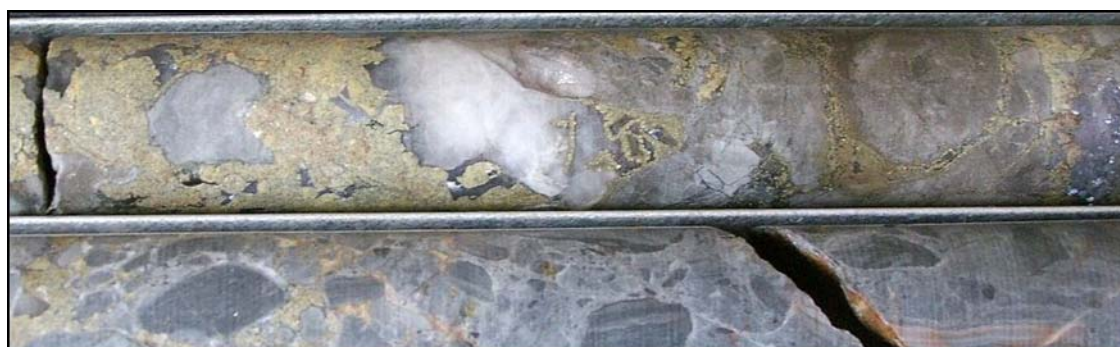
Figure 9 – Zinc sulphide (greenish) and lead sulphide (galena) from Border, a Berg Aukas-type deposit.
