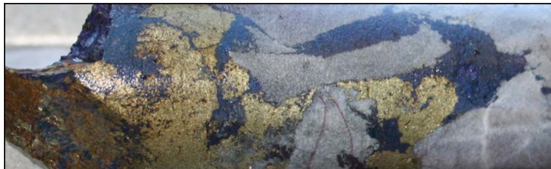
Figure 10 – The copper sulphides chalcocopyrite (golden) and bornite (violet) from a Tsumeb-type deposit.
