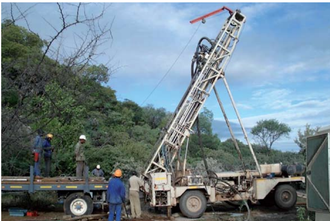
Figure 3 – RC drilling adjacent to Adit Hill, Border deposit.
