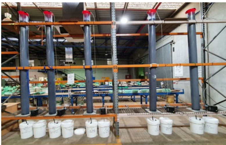
Plate 3 – Heap Leach column tests underway at Bureau Veritas in Canning Vale (March-April 2022).
