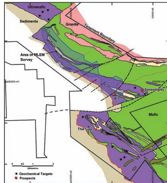
Figure 6. Geology plan of the Carlingup area showing targets and the MLEM survey position
